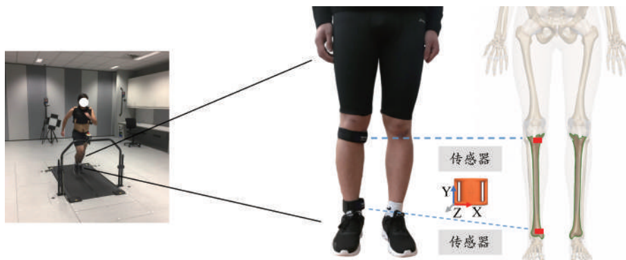
图 5 实验过程中传感器的放置位置 Figure 5. Placement of Sensors during the Experiment
